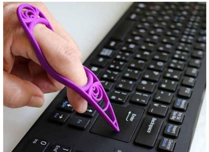
A tool to type on a key board without using (much) muscle strength (Halterman, T.E., 2015)
