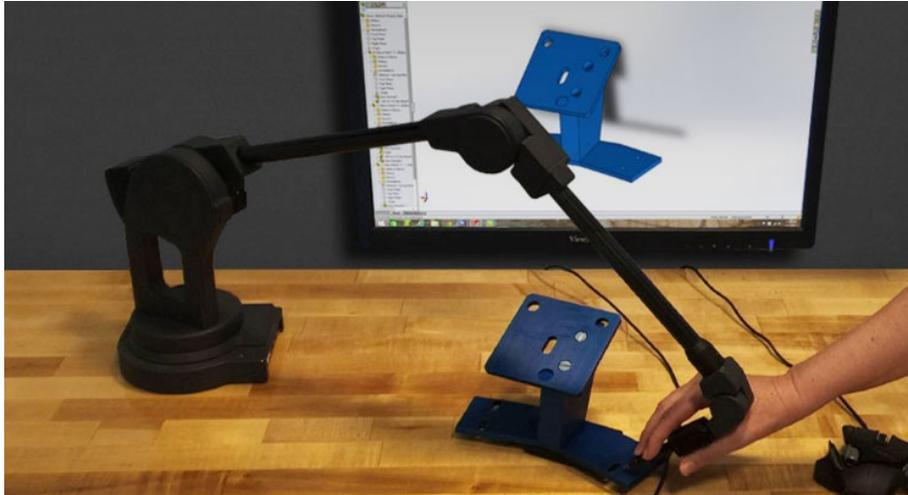
Another limitation of Laser 3D scanning is the Line of Sight. Given the optical nature of 3D laser scanning, it is impossible to measure any surface that is out of the scanner’s line of sight. This means that hidden or internal geometry that is not visible to the scanner is unable to be measured. Scans are taken from many different angles in order to ensure a complete model, but complex geometry may still prove to be a problem, such as commonly occurs with holes or threads.
