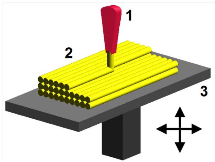
A heated nozzle (1) ejects molten plastic, depositing it in thin layers, one on top of another (2), onto a print bed (3), eventually forming the 3D printed part.
