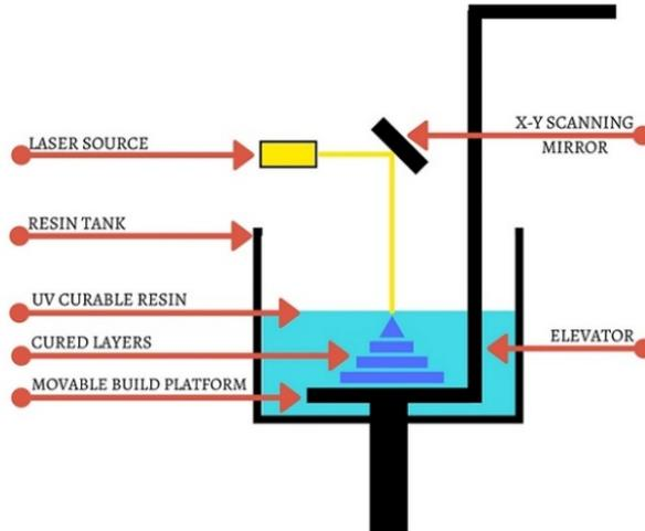
It works by using a high-powered laser to harden liquid resin that is contained in a reservoir to create the desired 3D shape. In other words, this process converts photosensitive liquid into 3D solid plastics in a layer-by-layer fashion using a low-power laser and photopolymerization.
