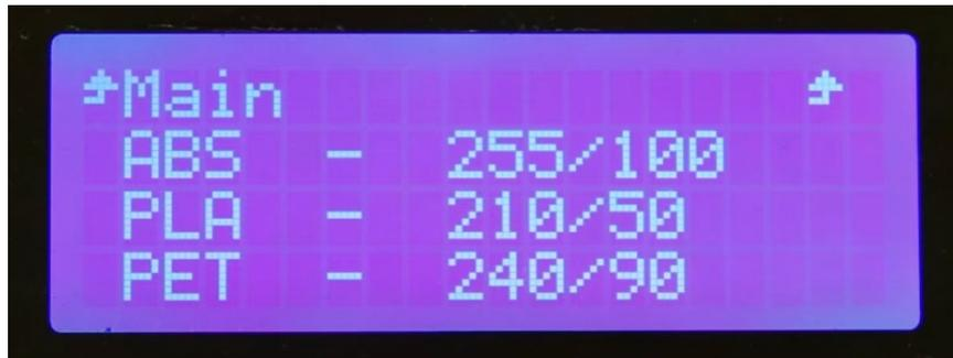
In the picture above, you can see examples of Preheat options for different materials. The first number states the required **hot end temperature**, while the second number states the required **Bed temperature**.
