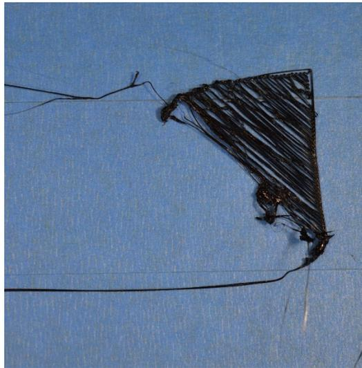
That is typically a sign that the nozzle is too far from the build surface. You have to make sure that the build surface is leveled, so you need to level the Bed as described in Exercise 2 and/or clean the Bed.
